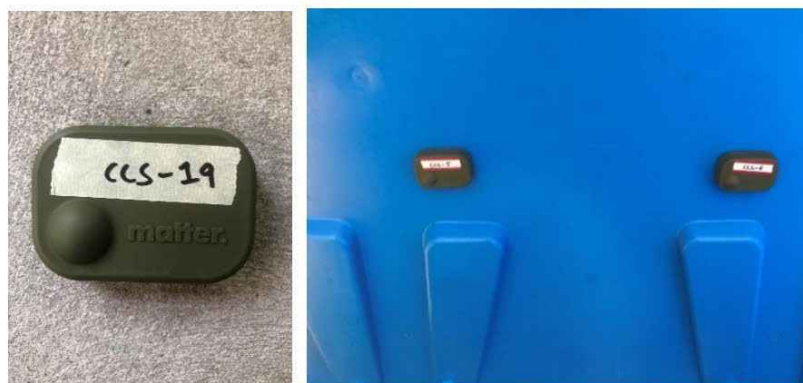
Figure 27: Sensors installed inside the bulk bin lid
