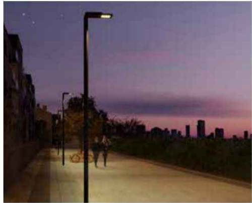
Light Pole We-ef AFL100 series Material - Aluminium Finish - Powdercoated (Black)
