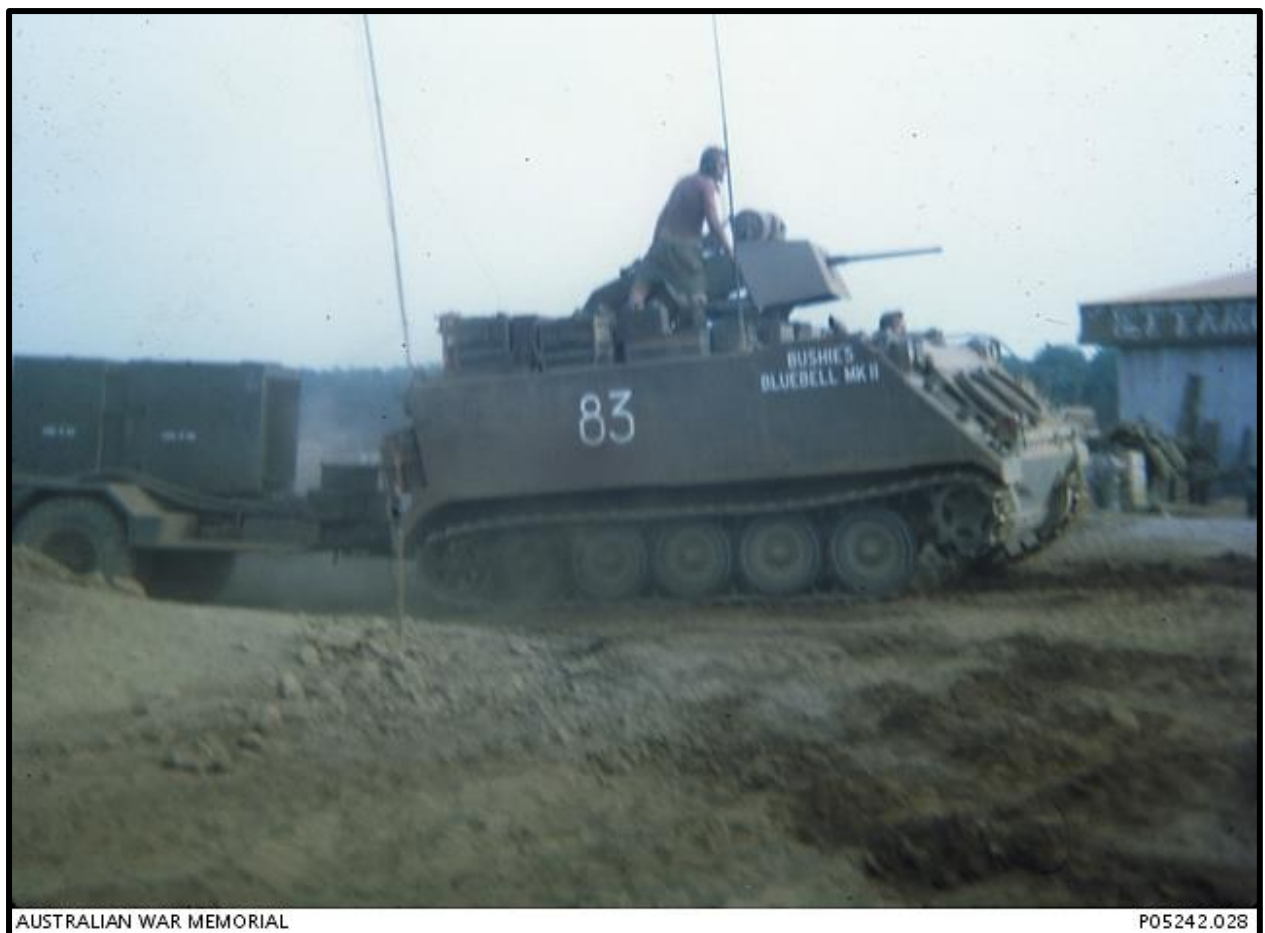
A 17 Construction Squadron, Royal Australian Engineers (RAE), M113A1 fitters vehicle named 'Bushies Bluebell Mk II' with the call sign 83 driving through the Night Defence Base (NDB) Garth. It is armed with an M2 .50 calibre heavy machine gun and is towing a trailer which may contain generators. [ https://www.awm.gov.au/collection/C1147869 ]
