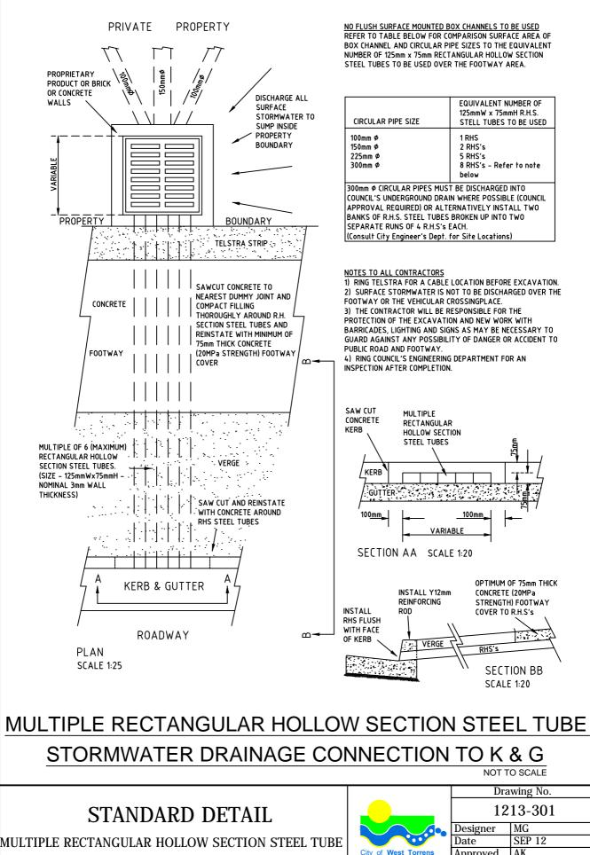
STORMWATER DRAINAGE CONNECTION TO K & G
