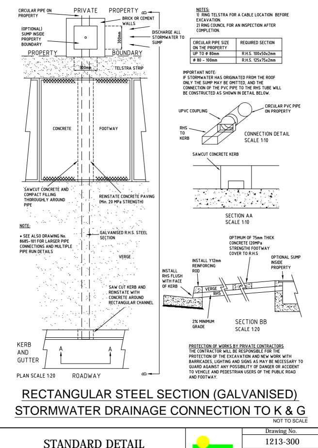
STANDARD DETAIL RECTANGULAR STEEL SECTION (GALVANISED) STORMWATER DRAINAGE CONNECTION TO K & G
