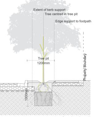
Section Detail 1:50 @ A4 Soil Volume Achieved: 5.9m3 Permeable Surface: 9.6m2
