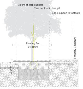
Section Detail 1:50 @ A4 Soil Volume Achieved: 3.4m3 Permeable Surface: 4.2m2
