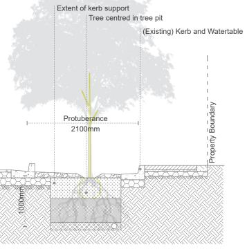
Section Detail 1:50 @ A4 Soil Volume Achieved: 2.7m3 Permeable Surface: 4.1m2
