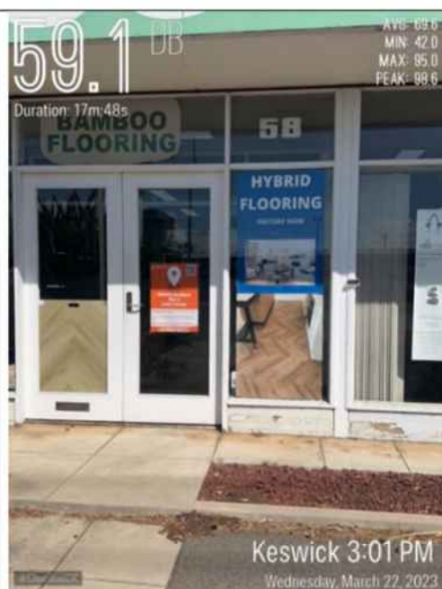
Measurement of DBSPL at front door, please note the higher SPL level is from traffic and ambient noise
