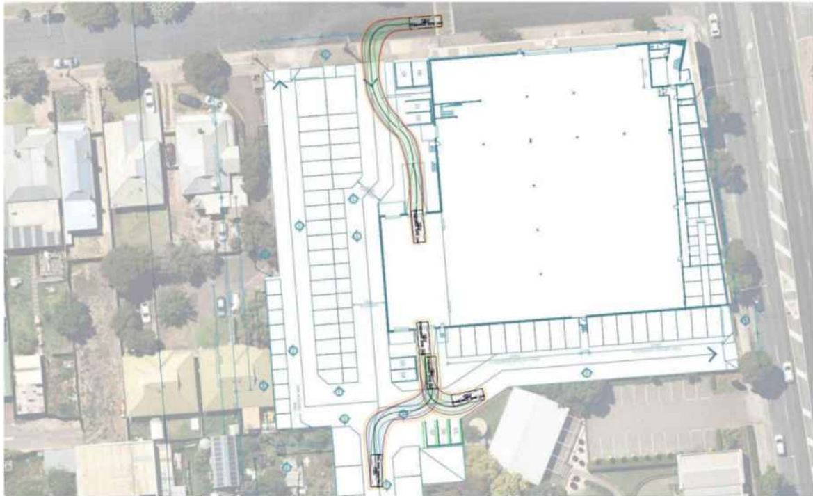
Figure 6: 6.4m SRV Building Access
