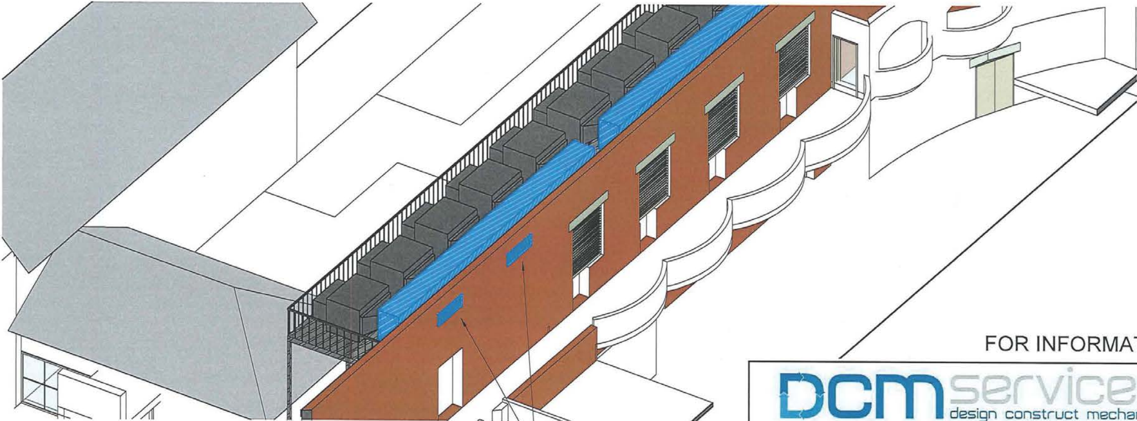
DOUBLE DEFLECTION SUPPLY AIR GRILLES ABOVE EXISTING WALL FEATURES
