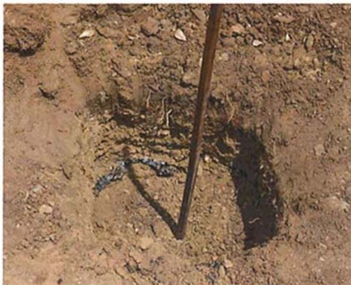
Example of the soil profile, showing bitumen and compacted road base in Miller Court garden. Material requiring complete removal and soil replacement ahead of planting
