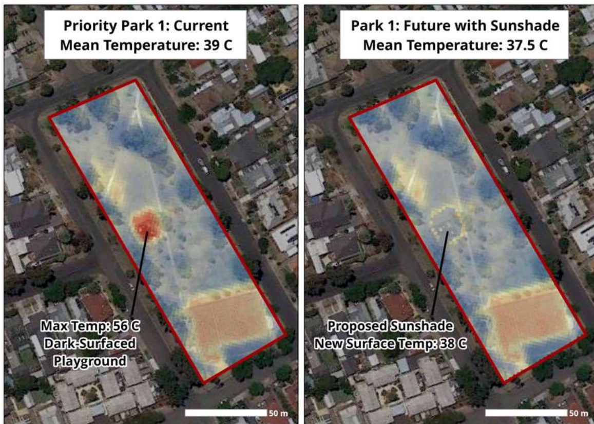
Figure 11. Results of prescriptive analysis for a playground where dark-surface covering is replaced in the thermal data set with a proposed sunshade.
