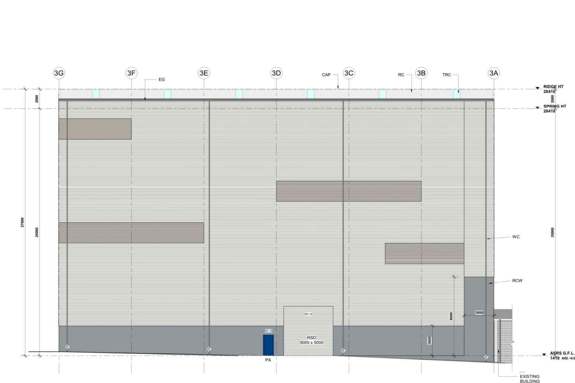
NORTH ELEVATION (ASRS BUILDING) 1 : 100 @ A1
