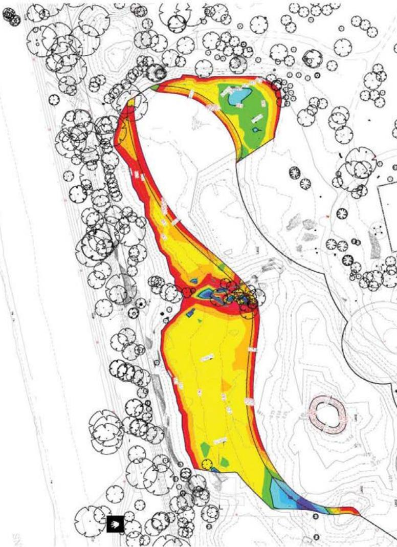
Figure 3 Fill depths required to create the Stage 2 wetland edge
