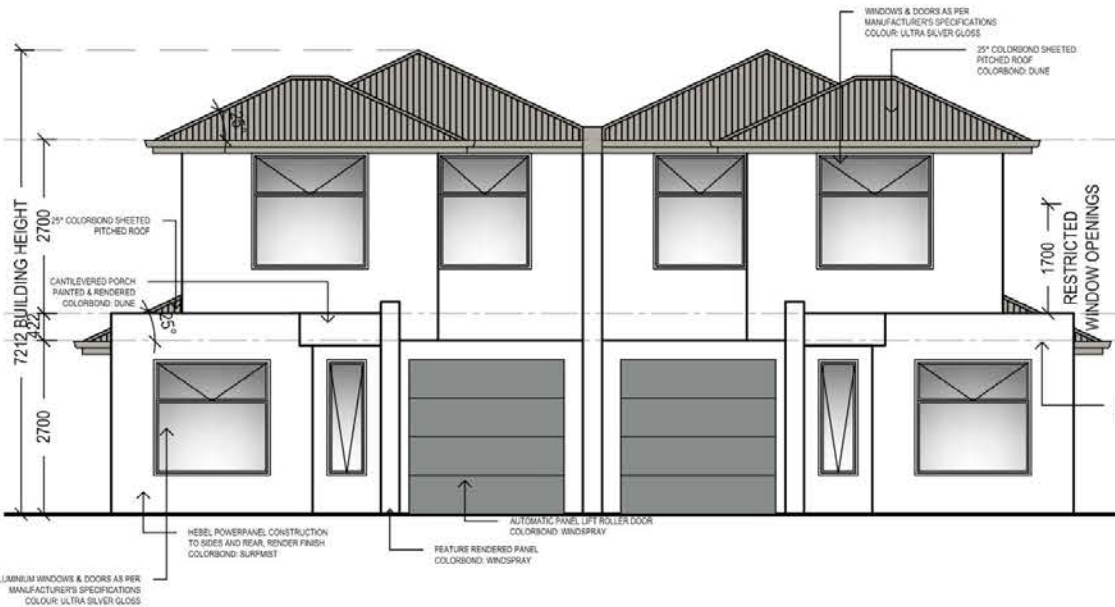
D3 - SOUTHERN ELEVATION SCALE 1:100
