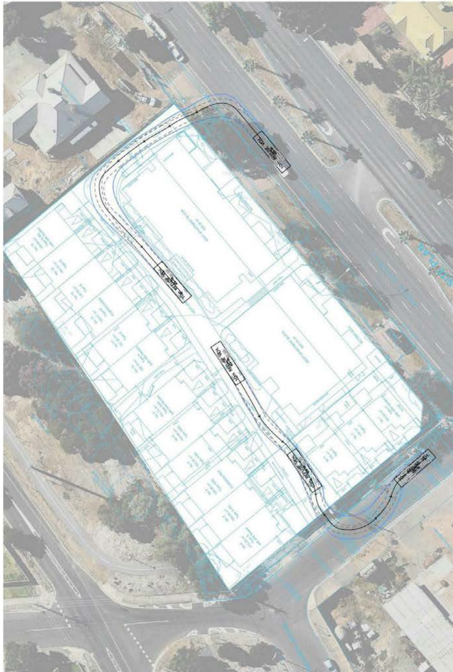
Figure 3 – Swept path modelling of 10m refuse truck from Anzac Highway to private lane and back onto Clifton St for collection of waste and recycling
