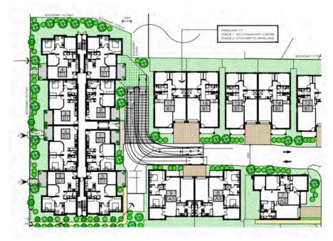
Above ground vehicle turning movements entering and exiting the ramp to the undercroft car park
