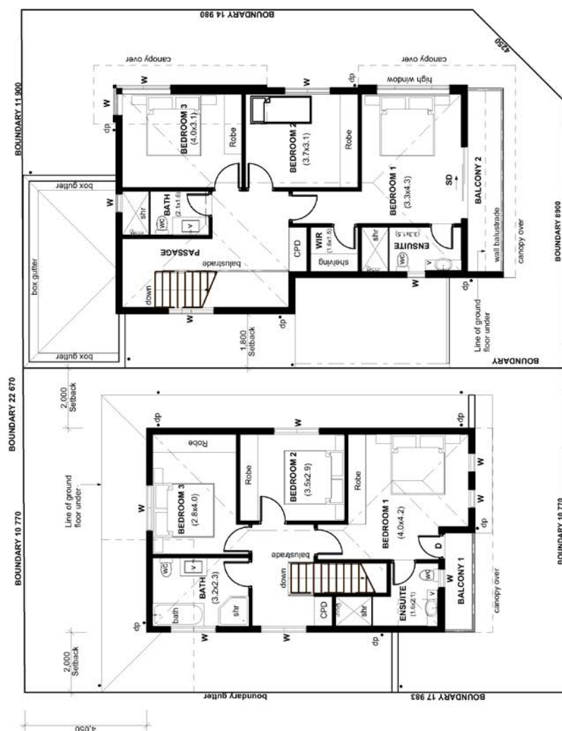
Proposed Upper Floor Plan 1:100
